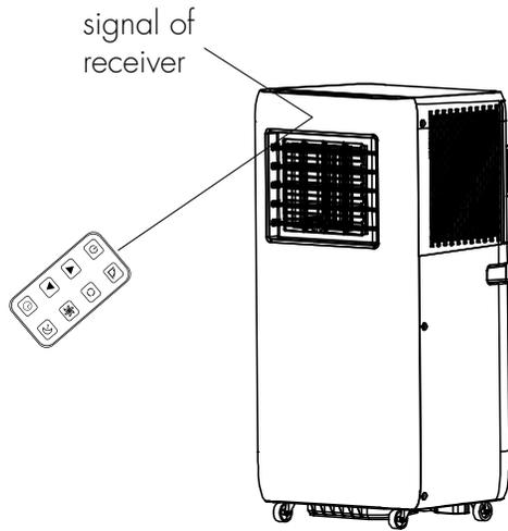
Make sure to direct the remote controller towards the signal receiver located on the front of the appliance, as shown in the figure.
